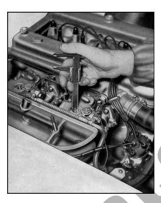
Checking the fuel level in the float chambers with the carburettors on the car
